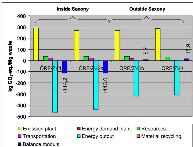
Figure 8: Climate effects of waste management in the Free State of Saxony 2006 – here: Incineration solutions realized in three waste management areas (ÖRE/ZV) [BIWA/BZL/Prof. Born 2009] – results referring to 1 Mg residual waste
