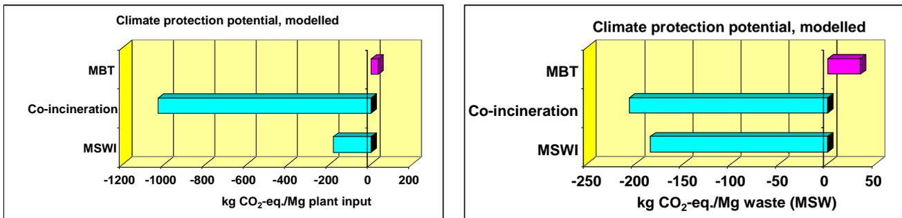
Figure 2: Results of the study by Öko-Institut (2005) based on 1 Mg plant input (left) and 1 Mg municipal waste (right) (without credits for separated metals) [Zeschmar-Lahl 2009]
