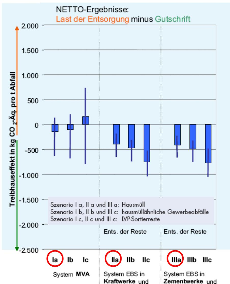
Figure 5: Climate effects of waste management in the North Rhine-Westfalia [Fehrenbach et al. 2007] – results referring to 1 Mg residual waste (I), commercial waste similar to household waste (II) and residues of sorting of lightweight packaging (III)
