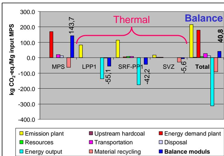
Figure 6: Climate effects of waste management in the Free State of Saxony 2006 – here: MPS + energy/material recovery [BIWA/BZL/Prof. Born 2009] – results referring to 1 Mg residual waste (input in MPS)
