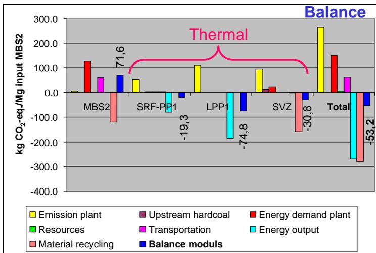
Figure 7: Climate effects of waste management in the Free State of Saxony 2006 – here: MBS + energy/material recovery [BIWA/BZL/Prof. Born 2009] – results referring to 1 Mg residual waste (input in MBS)
