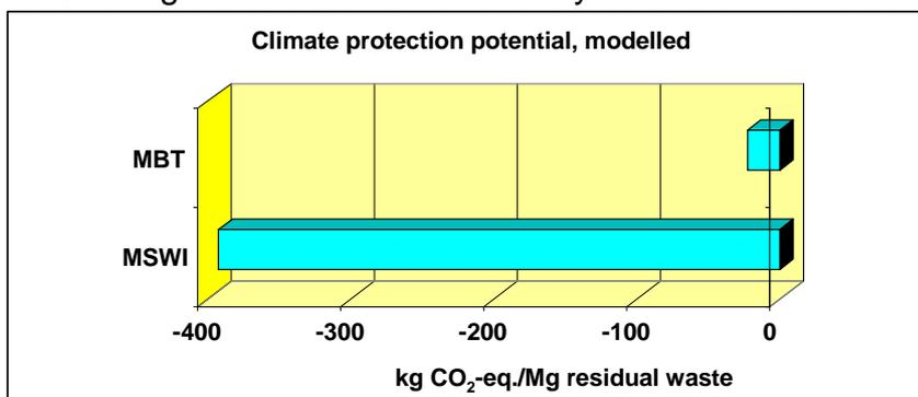
Figure 4: Climate effects of waste management in the Free State of Bavaria [Peche et al. 2007] – results referring to 1 Mg residual waste
